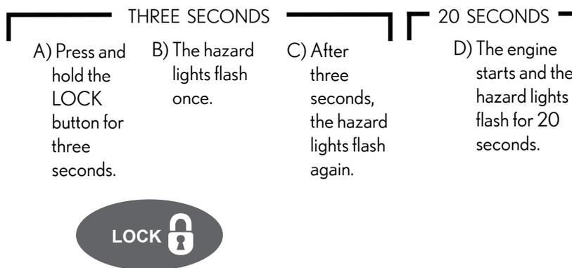
**NOTE:** Vehicles started with the Remote Engine Starter can idle for a total of 20 minutes, however automatic engine shutdown occurs after 10 minutes of run-time. You can always restart the Vehicle after this initial shutdown. Once the total run-time exceeds 20 minutes the vehicle must be manually started in order to reset the Remote Engine Starter.
